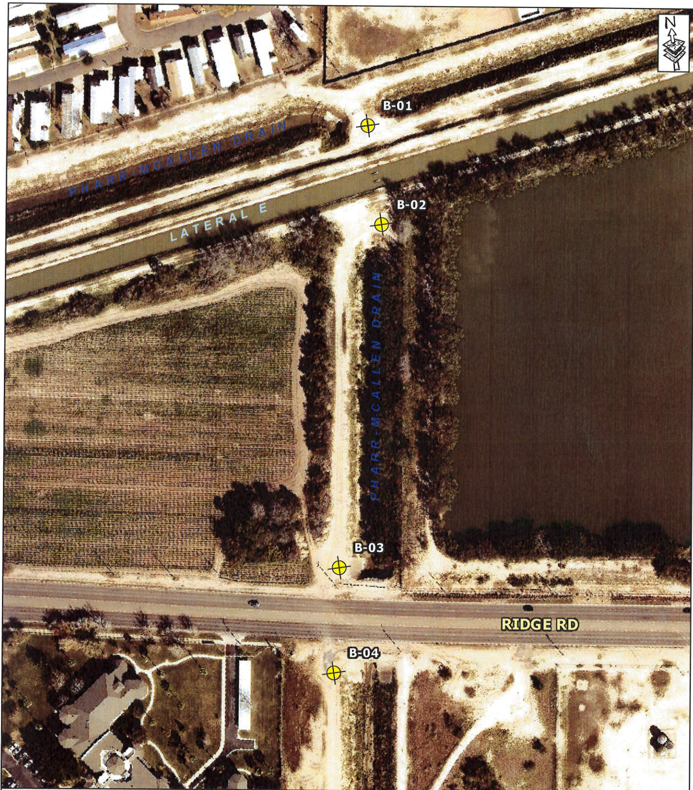
Figure 2 HCDD #1 Pharr-McAllen Drain Boring Location Map
